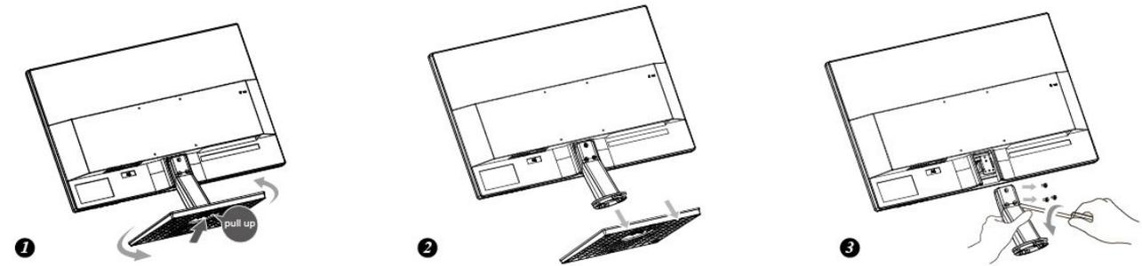
Figure.1. Installing and Removing the Base
