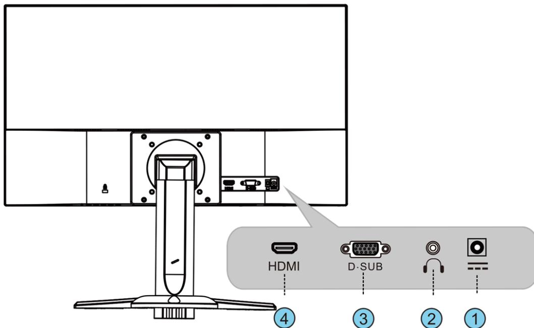
Figure.2. Connecting to a PC
