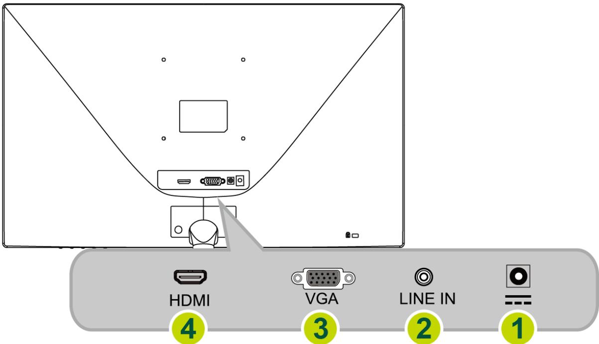
Figure.2. Connecting to a PC
