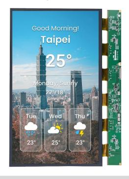
The HSD215GUW1-90000A-MX is a color active matrix thin film transistor (TFT) liquid crystal display (LCD) that uses amorphous silicon TFT as a switching device.
